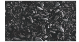
Perio-Mate Powder (glycine) Average particle diameter: 25 µm Scanning electron microscope image magnification of 150 X
